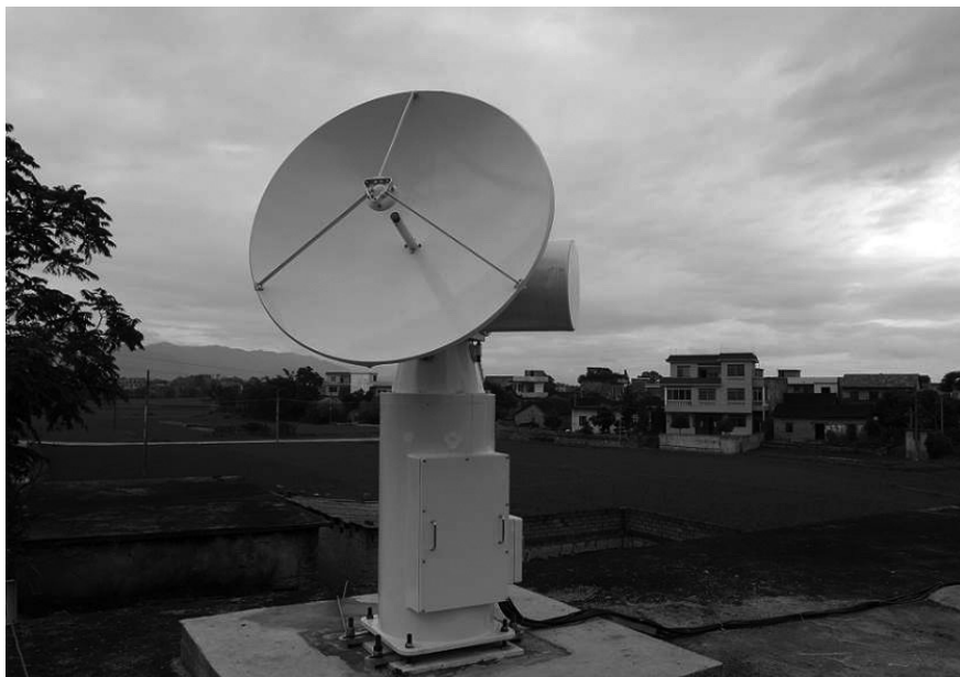
Fig. 16.4. The millimetric scanning entomological radar developed by the Institute of Plant Protection of the Chinese Academy of Agricultural Sciences (CAAS-IPP).
